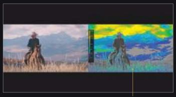
HDR Metering shown. Works both with SMPTE 2084 (PQ) and Hybrid Log-Gamma (HLG).
