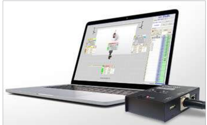
DMX Bridge connected to computer for lighting control
