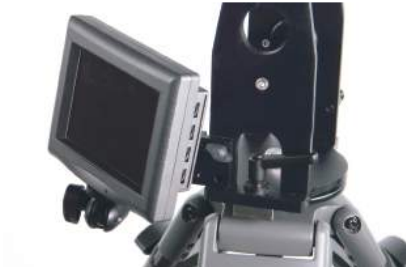
FIG 64. Add the monitor to the ball head and lock it off to desired position.
