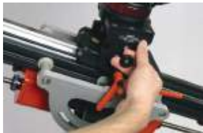
FIG 32. While holding the camera, pull out the black circular adjustment knob and position the camera in a level or desired position.
