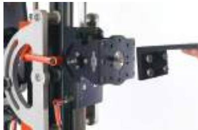
FIG 59. To mount the right angle plate, line the holes on the short side of the plate with the hole pattern on the slider platform.
