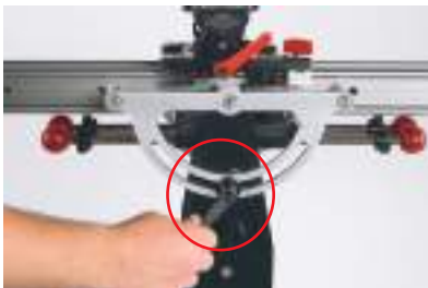
FIG 7. Secure the rail system with the two black 'kip' handles.
