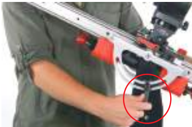
FIG 29. Tighten the black 'kip' handles on each side of the fulcrum head.
