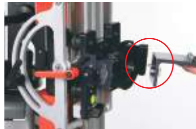
FIG 69. To mount the right angle plate, line the holes on the short side of the plate with the hole pattern on the slider platform.
