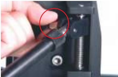
FIG 45. Install the end of the parallelogram arm opposite the small lever with the red 'kip' handle onto the focal point adjustment located on the fulcrum head.
