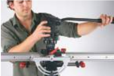
FIG 9. Tighten the flat plate fluid head to the rail platform until it is secure.
