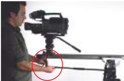
FIG 47. Attach the opposite side of the parallelogram arm to the camera platform by inserting the red 'kip' handle bolt into the threaded hole.
