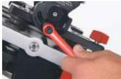
FIG 30. Hold the camera with one hand and loosen the red 'kip' handle under the black circular adjustment knob.
