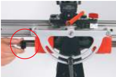
FIG 13. Reattach the black nuts for weight security.
