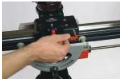
FIG 16. Loosen the red slider brake.
