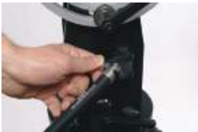
FIG 45. Install the end of the parallelogram arm opposite the small lever with the red 'kip' handle onto the focal point adjustment located on the fulcrum head.
