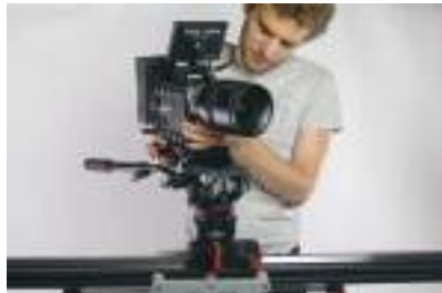
FIG 12. Mount your camera package to the fluid head (camera package and fluid head not to exceed 32kg).
