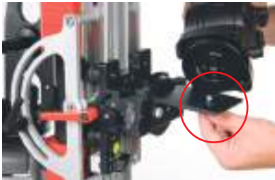
FIG 71. Mount your flat plate fluid head to the top of the right angle plate using the screw provided.
