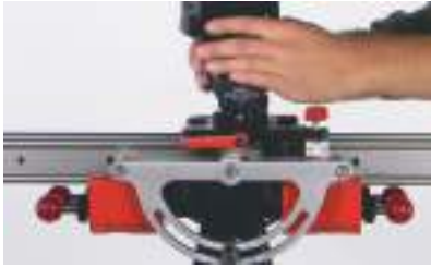
FIG 25. To angle the rail for diagonal slides, move the camera to the middle of the rail.
