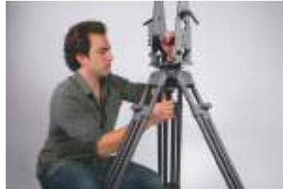
FIG 2. Insert the fulcrum head and level it accordingly.
