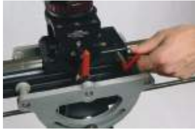
FIG 10. Loosen the red slider brake.
