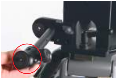
FIG 63. Mount your ball head of choice to the 1/4" end of the rod.
