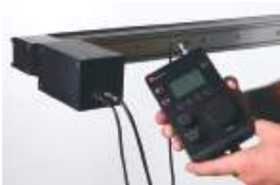
FIG 76. The stepper motor is operated with a microprocessor, allowing the user to operate the slider and tower configurations. Time lapse, manual movement and programmable repeated movements are possible with the use of these accessories.
