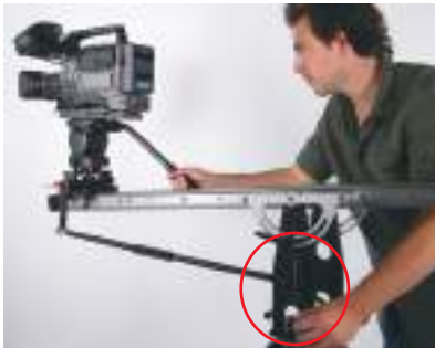
FIG 57. Loosening up the fulcrum brake handles will allow 360 degree rotations around the vertical access of the tripod.
