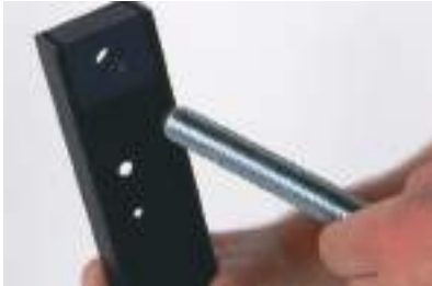
FIG 36. Insert the threaded platforms into the feet.
