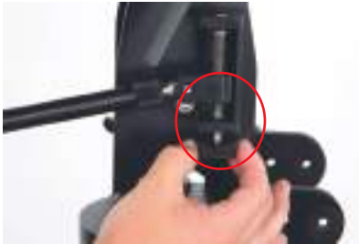
FIG 55. If you desire to keep an object within the camera frame, reposition the focal point adjustment to the bottom.
