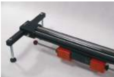
FIG 36. Insert the feet to each end of the rail.
