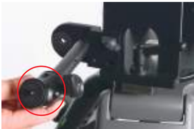
FIG 66. Mount your ball head of choice to the 1/4" end of the rod.
