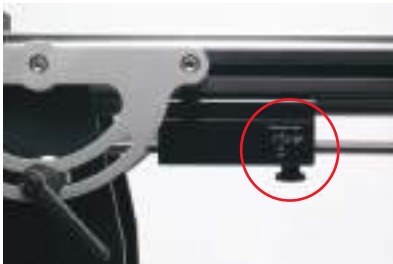
FIG 11. Loosen the safety lock and move the dolly to the middle of the rail. Then lock the dolly using the red slider brake.
