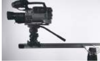
FIG 42. With both black 'kip' handles tightened on each side of the fulcrum head, slide the camera package to the end of the rail opposite the crank spline.
