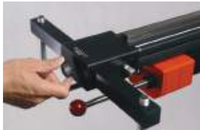
FIG 37. Lock the feet using the screws provided.
