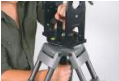
FIG 3. Secure the fulcrum head using the long black handle with female threaded hole.
