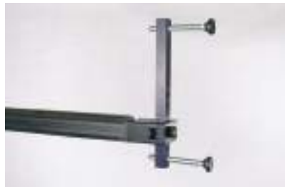
FIG 56. Add one of the feet with the threaded platforms to the side opposite the crank spline. Make sure the long side of the foot is facing outward.
