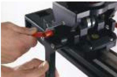
FIG 45. Install the end of the parallelogram arm opposite the small lever with the red 'kip' handle onto the focal point adjustment located on the fulcrum head.
