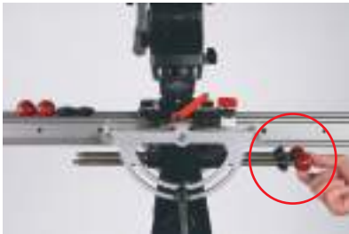
FIG 11. Remove the black nuts and the red protective balls from the counterbalance sled.
