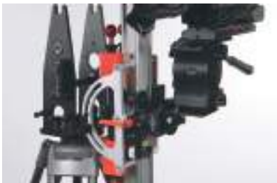
FIG 72. Mount your camera package to the fluid head to complete vertical tower configuration.
