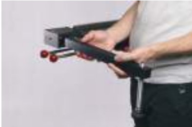
FIG 36. Insert the feet to each end of the rail.
