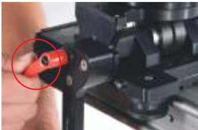
FIG 51. Complete tightening process with the red 'kip' handle. Ensure the teeth in the middle of the camera platform are fully disengaged and that the nipples on the arm's lever have fully met the holes on the platform.
