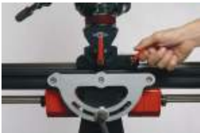
FIG 27. Apply the red slider brake handle.
