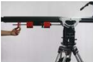
FIG 21. You may need to add or subtract counterbalance weight for precision. Repeat steps 13-20 if rebalancing is needed.
