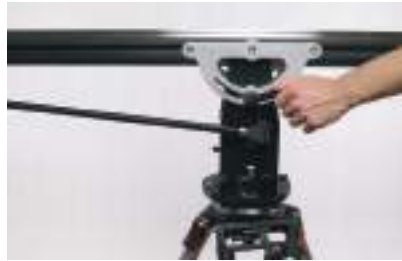
FIG 50. Release the black 'kip' handles on each side of the fulcrum head to activate the mini jib function.
