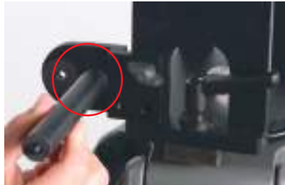
FIG 65. Attach the black mounting rod by screwing it onto the ear.
