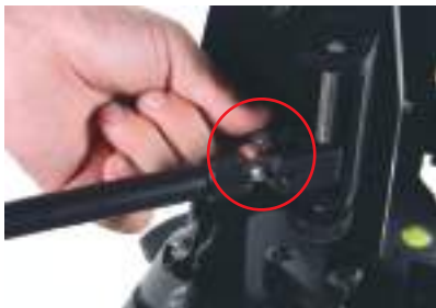
FIG 60. Once the parallelogram arm has been removed from the camera platform side, remove the opposite end on the fulcrum head.
