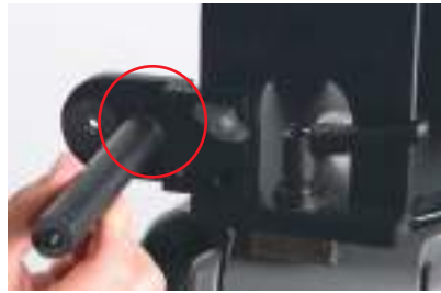
FIG 62. Attach the black mounting rod by screwing it onto the ear.
