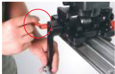
FIG 48. The lever with red 'kip' handle should be perpendicular to the rail. This will ensure parallel camera movement to the ground.
