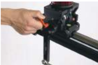
FIG 53. Remove the parallelogram lever by releasing the red 'kip' handle.
