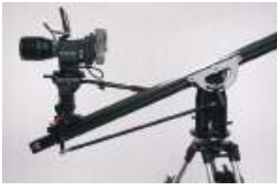
FIG 51. As the mini jib moves up and down, the camera should stay parallel with the ground. Loosening up the fulcrum brake handles will allow 360 degree rotations around the vertical axis of the tripod.
