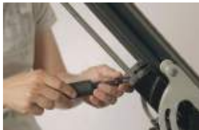
FIG 73. Grease the counterweight bearings using the grease gun provided.
