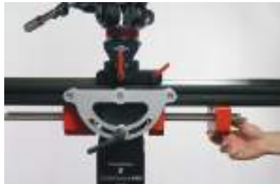
FIG 14. Add counterweight to the sled to equal the weight of the camera and fluid head package.
