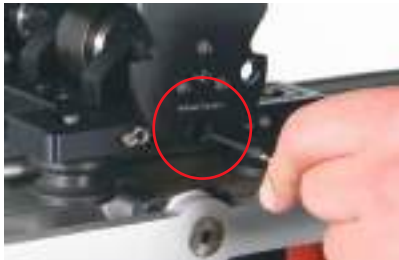
FIG 77. The wheel tension is set by the manufacturer. With time and frequency, it may be necessary to adjust the tension with the M2.5 allen key provided in the system.
