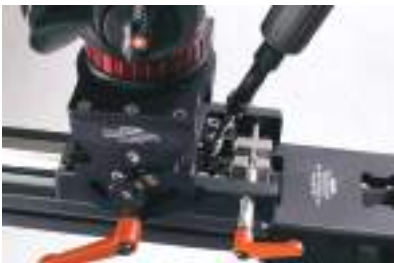
FIG 72. Grease the dolly bearings using the grease gun provided.
