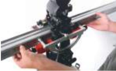
FIG 41. Level the rail and the counterbalanced fluid head and camera package.
