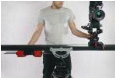
FIG 17. Slide the camera away from the center.
