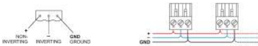
Figure 8. Balanced analogue input pin-out (left) and daisy-chaining cables in the analogue input Euroblock connector (right).
