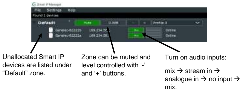
Figure 9. Controlling the zone with Smart IP Manager software.
