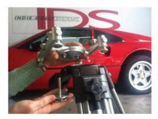
In order to mount a section of IDS Slider "plus" track onto a tripod, you need a tripod with a 100mm bowl.
