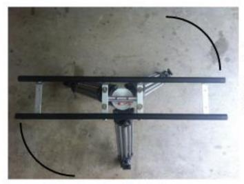
You can rotate the track section in order to tighten the bolt on the bottom even more.
