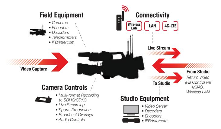
The system features the real-time integration of ground-breaking technologies, such as bidirectional camera operator communication (return video via IP, IFB via MIMO Wireless LAN) with a central control center (GPS, status, camera control), online post-production systems (native file progressive FTP), and live IP distribution networks (live VoIP and data transport).
