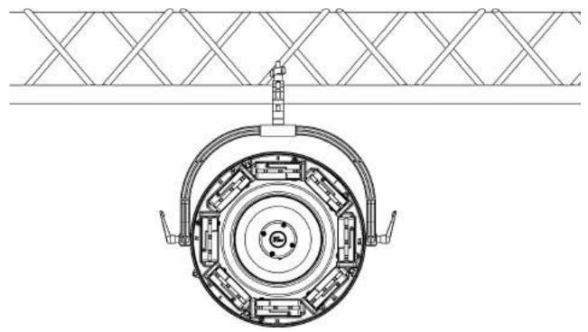
You can also fasten the product on a horizontal rigging structure:
