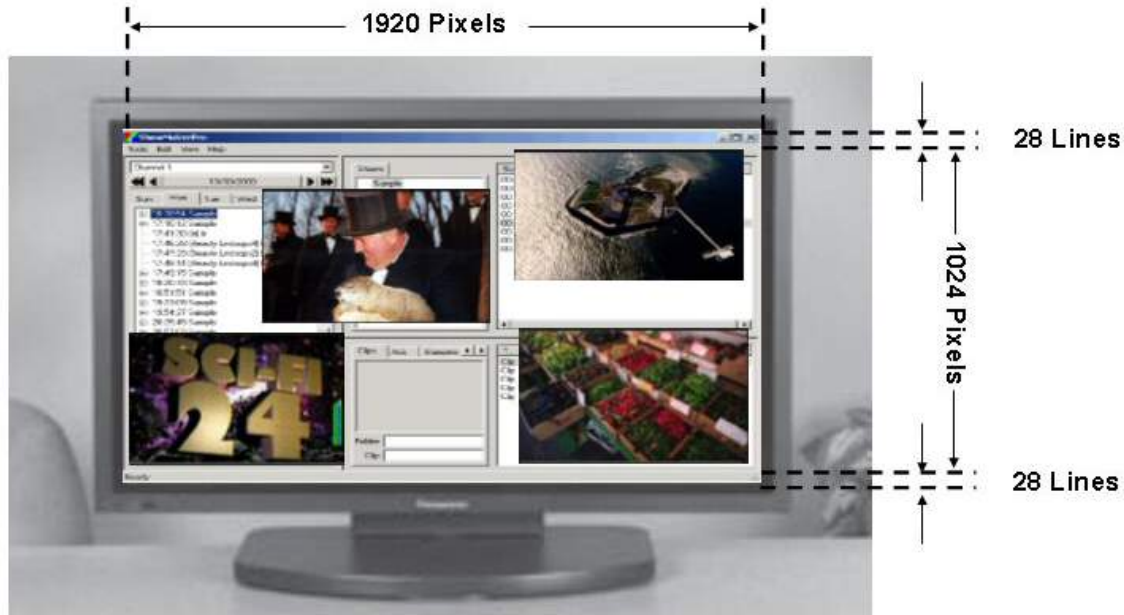
Figure A2 Kaleido-Quad output on a 1920x1080 display showing the DVI background occupying the entire display with the Kaleido layout elements keyed in.
