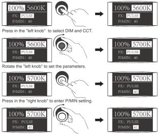
Rotate the "right knob" and set the P/MIN.
