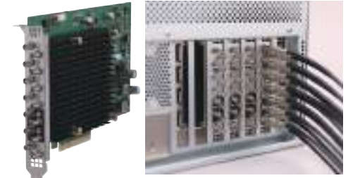
AT-KC20M1 SDI input/output board and its installation example
