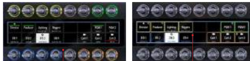
Assign group colors to the LED rings or on the key labels
