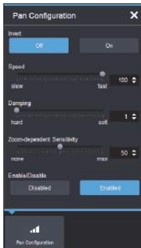
Figure 12 - Axis Configuration dialog box (pan configuration shown)
