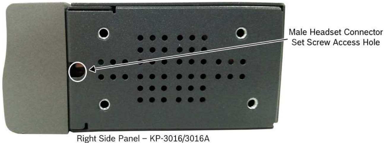
FIGURE 6. Male Headset Connector Set Screw Access Hole
