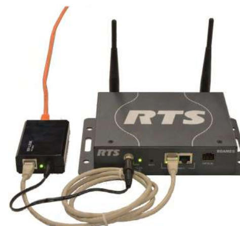
Figure 3. How to connect the PoE adapter
