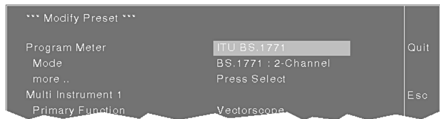
Fig. E 5-7: The Modify Preset menu, when ITU BS.1771 mode is selected
