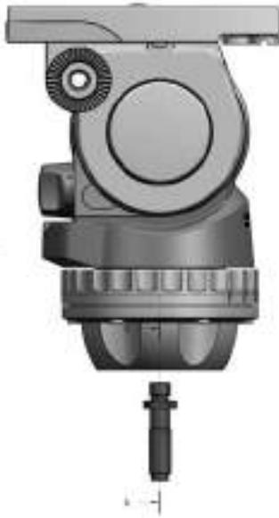
If you want to fit the FSB 4 onto a flat base, remove the threaded pin.
