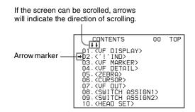
Rotate the MENU SEL knob/ENTER button to align the arrow marker (→) with the desired page indication, then push on the MENU SEL knob/ENTER button.
