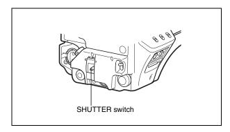
The current shutter setting will be displayed in the setting change/adjustment progress message display area of the viewfinder screen for about three seconds.
