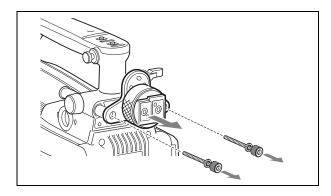
**3** Using the two bolts  $(M4 \times 8)$  and the washers removed from the camera in step **2**, attach the rotation mechanism assembly of the BKW-401 to the camera.
