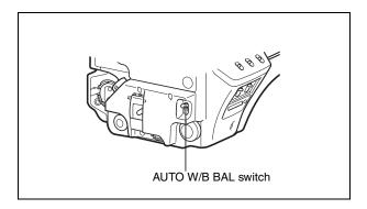
The switch will return to the center position, and adjustment will be performed.
