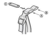
2 ① Remove the back screw-hole cover on the top of the camera and ② secure the cable clamp belt to the camera, using the two supplied screws (+B3×10).
