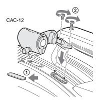
2 Loosen the screw to open the CAC-12 and attach the microphone.
