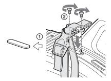
3 ① Release the buckle, ② bundle the cable with the belt, ③ then lock the buckle again.
