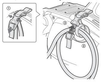
4 Adjust the length by pulling down the end of the belt.
