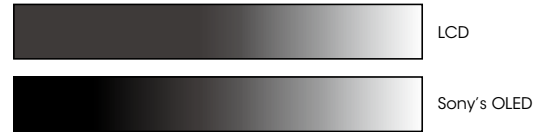
Grey scale images corresponding to the input signal * Grey scales are simulated images.
