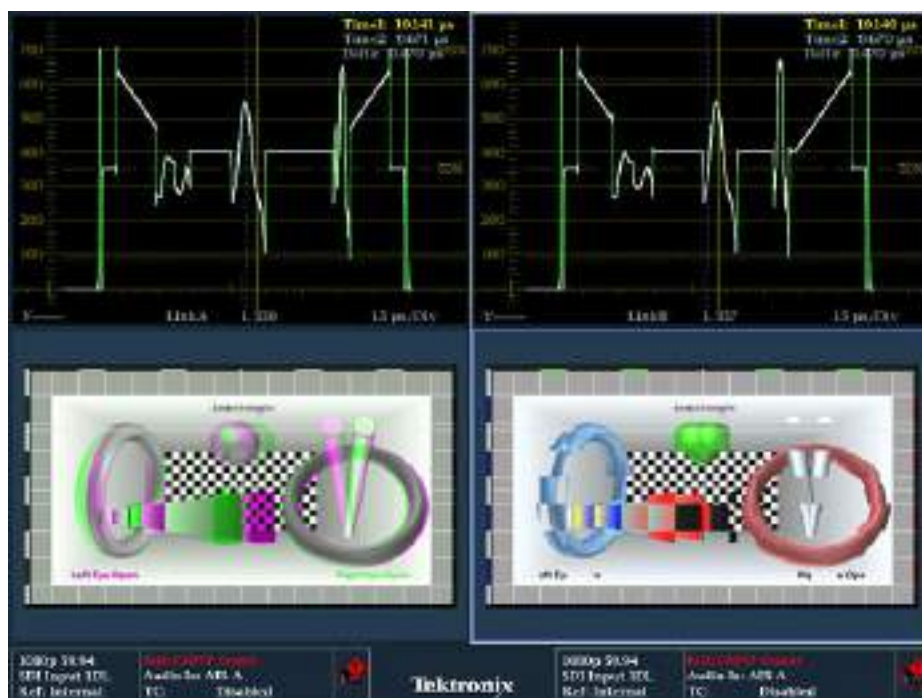
Figure 14: 3D Left and Right Eye images showing Green/Magenta Anaglyph and Checkerboard display using SIM
